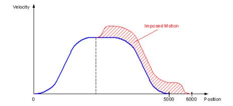
For example, when a scanning camera performs a capture and calculates its position while the axis is still in motion. A superimposed motion is executed, changing the camera end position on-the-fly. A newly calculated position, velocity and AC/DC is added to the ongoing motion.
