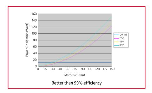
As a result of the high efficiency and "High Quality" power dissipation, the temperature rise is very slow and under full control. In fact, this scenario can maintain 150 A consumption for 500 seconds with an average current consumption of 100 A – 120 A. This is
