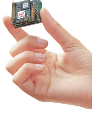
The Gold Twitter is a tiny, highly intelligent, high-powered servo drive. Weighing only 20grams, the Gold-Twitter is the ideal servo drive to be mounted anywhere: right on the motor, on moving axes, or within robotic joints. Its unparalleled power density is possible due to Elmo's proprietary and innovative Fast and Soft Power Switching Technology (FASST), resulting in over 99% efficiency and negligible EMI.
