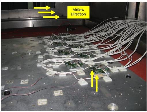
One accelerometer sensor was attached to the Jig Plate and one-on the Card of one unit
