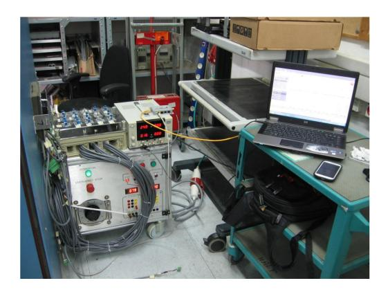
The **Set Up** included 10 servo drives G-TWI25/100EE (GOLD Twitter, 25A continuous, 50A peak, operating voltage range 10VDC to 96VDC)
