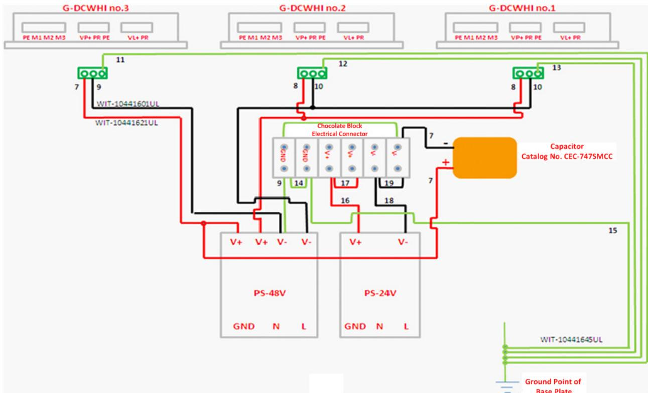
Figure 9: Mini Etude Connection Diagram
