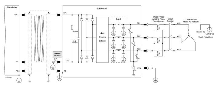
Figure 12: Three-Phase Isolated Source Connection
