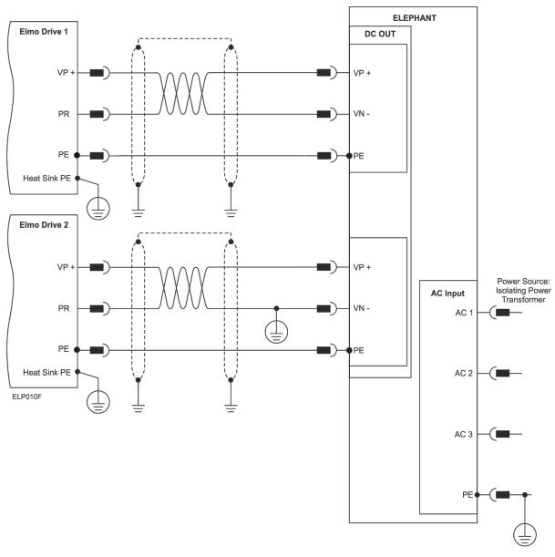
**Figure 13: Multiple Isolated Source Connection**
