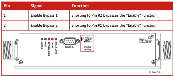
The Enable function in the Control connector can be ignored (if necessary) by connecting an isolated jumper between the two terminals of the "Enable Bypass" connector.
