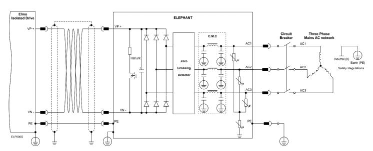
Figure 10: Three-Phase Direct-to-Mains Connection
