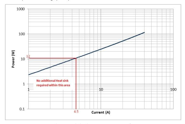
Figure 14: Dissipation versus Current Graph
