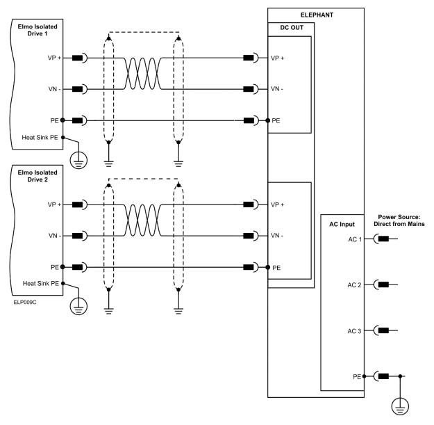
Figure 11: Multiple Direct-to-Mains Connection
