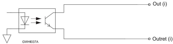
Figure 22: Digital Output Schematic
