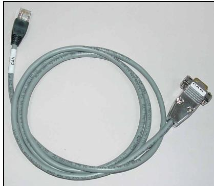
Figure A-5: CAN Cable (Part No. CBL-RJ45CAN1)
