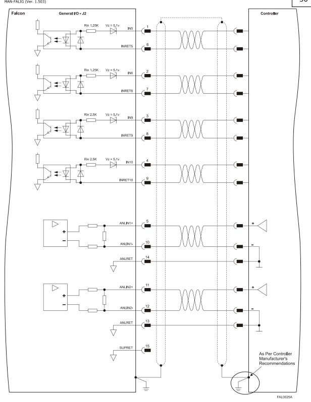
Figure 24: General Input J2 Connection Diagram
