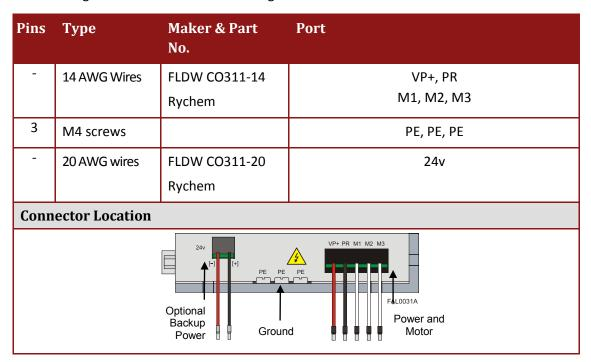
**Table 17: Connectors on the Bottom of the Falcon**
