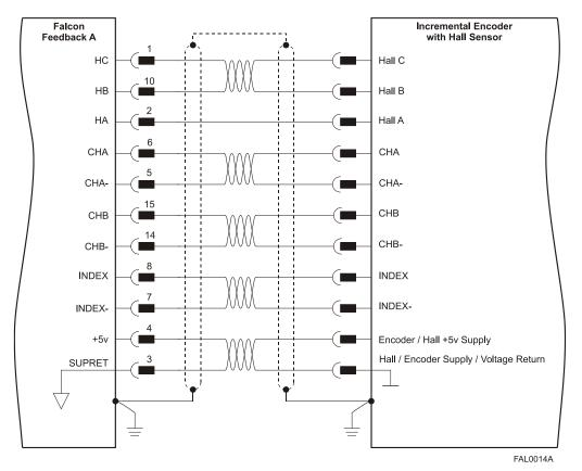
Figure 9: Main Feedback - Incremental Encoder Connection Diagram
