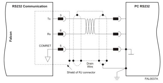
Figure 25: RS-232 Connection Diagram
