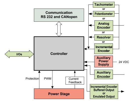
Figure 1: Falcon System Block Diagram
