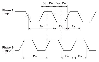
Figure 27: Encoder Phase Diagram
