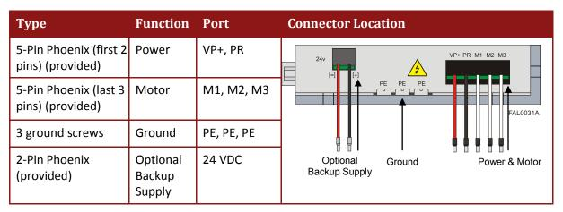
Table 1: Connectors on the "Bottom" of the Falcon
