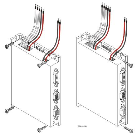
Figure 3: Mounting the Falcon
