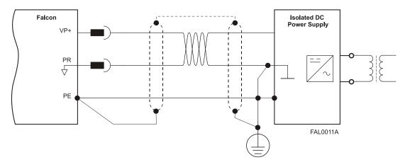
**Figure 6: Main Power Supply Connection Diagram**
