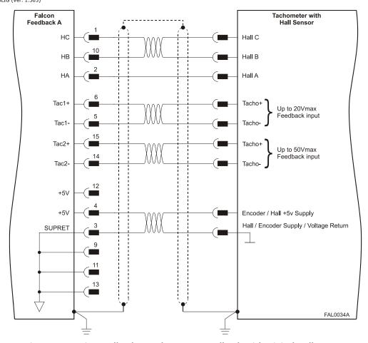
Figure 12: Main Feedback – Tachometer Feedback with Digital Hall Sensor Connection Diagram for Brushless Motors
