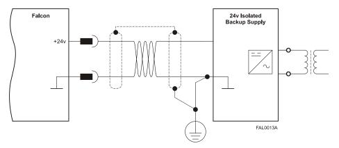
Figure 7: Backup Supply (24 V) Connection Diagram
