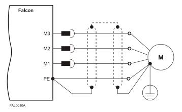
**Figure 5: AC Motor Power Connection Diagram**
