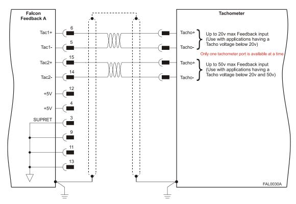
Figure 13: Main Feedback - Tachometer Feedback Connection Diagram for Brush Motors
