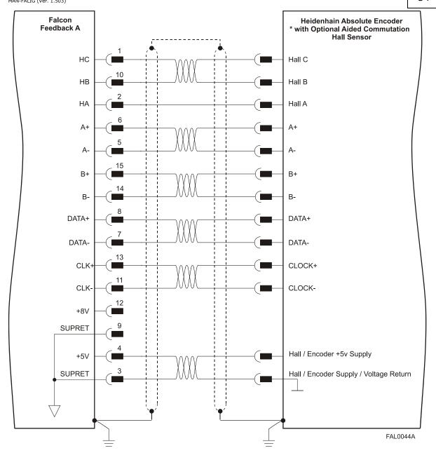
Figure 17: Main Feedback – Heidenhain Feedback Connection Diagram
