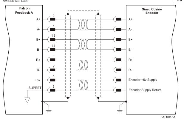
Figure 10: Main Feedback - Interpolated Analog (Sine/Cosine) Encoder Connection Diagram
