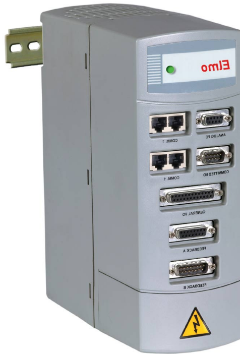
Figure 6: Tuba Mounted on a DIN Rail
