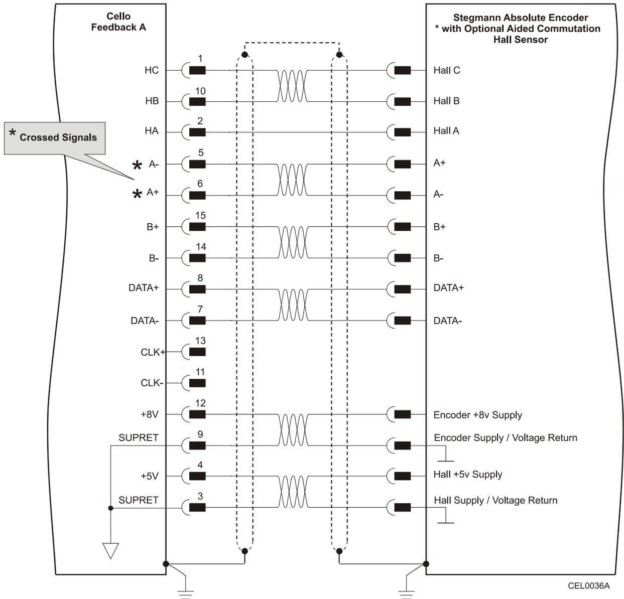
**Figure 16: Main Feedback – Stegmann Feedback Connection Diagram**
