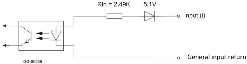
Figure 28: Digital Input Schematic
