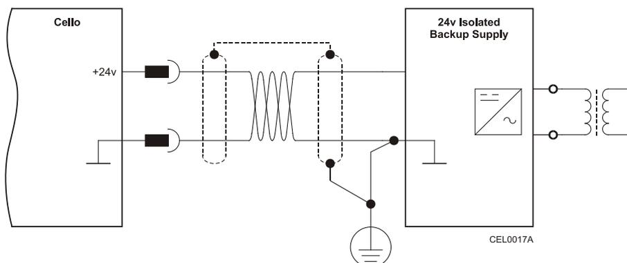
Figure 7: Backup Supply (24v) Connection Diagram
