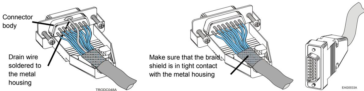
Figure 8: Feedback and Control Cable Assemblies
