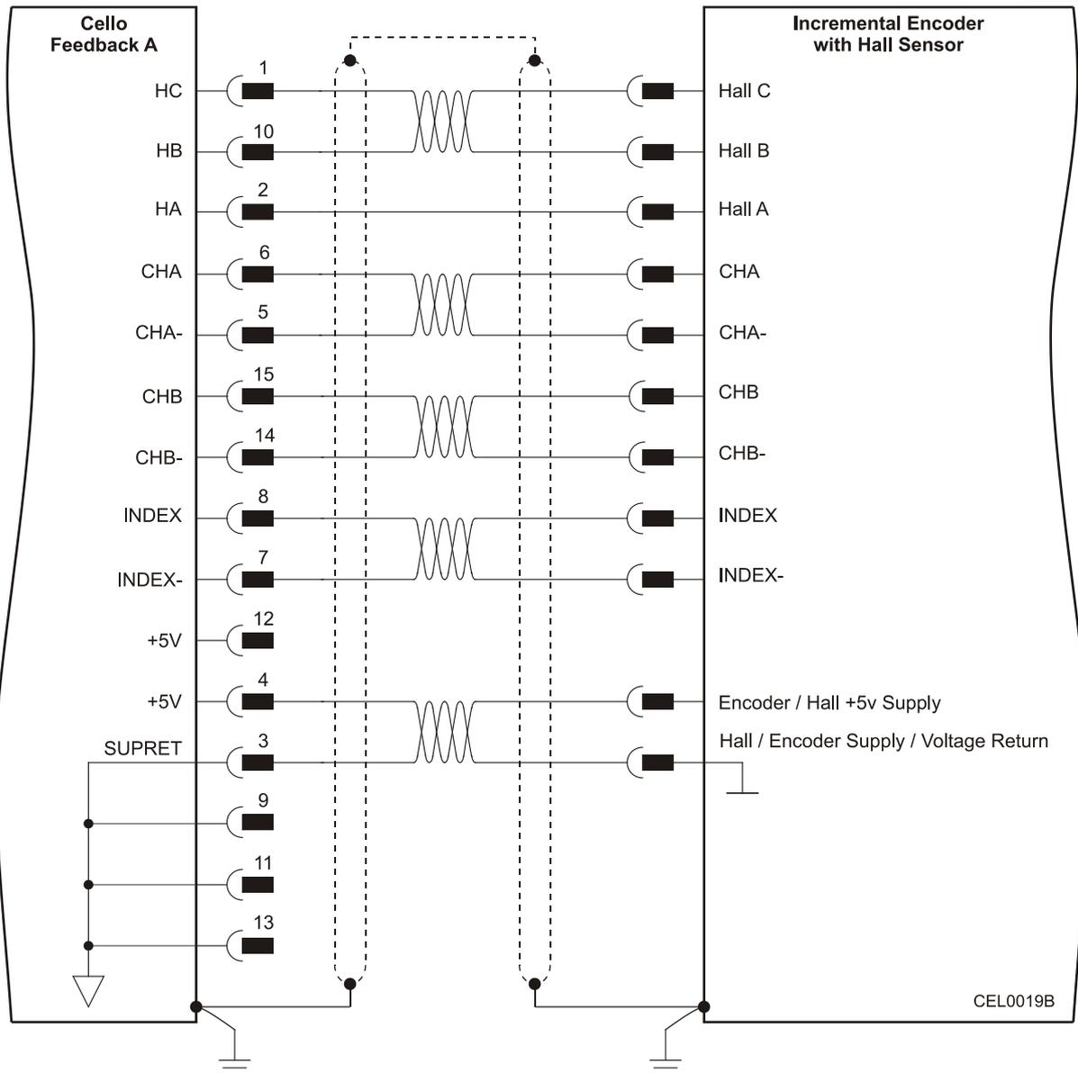
**Figure 9: Main Feedback- Incremental Encoder Connection Diagram**
