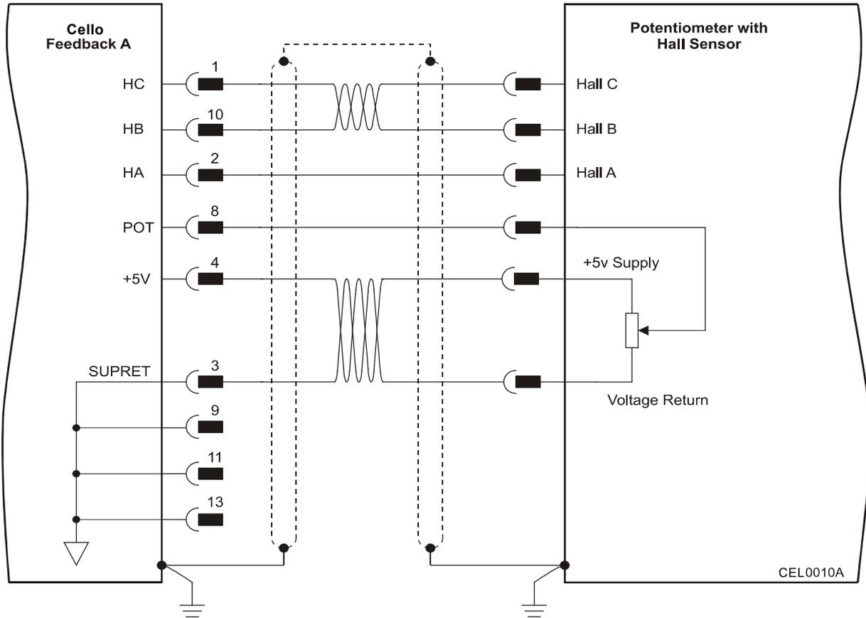
**Figure 14: Main Feedback – Potentiometer Feedback with Digital Hall Sensor Connection Diagram for Brushless Motors**
