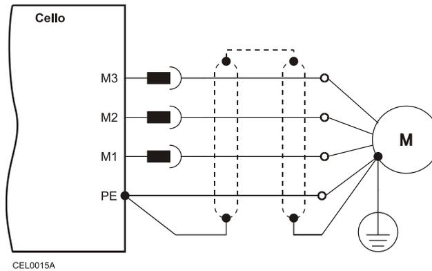
**Figure 5: AC Motor Power Connection Diagram**
