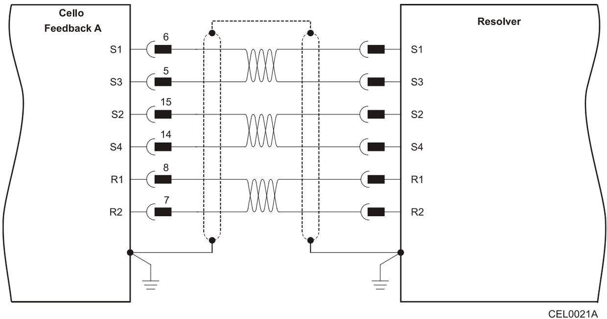
**Figure 11: Main Feedback – Resolver Connection Diagram**
