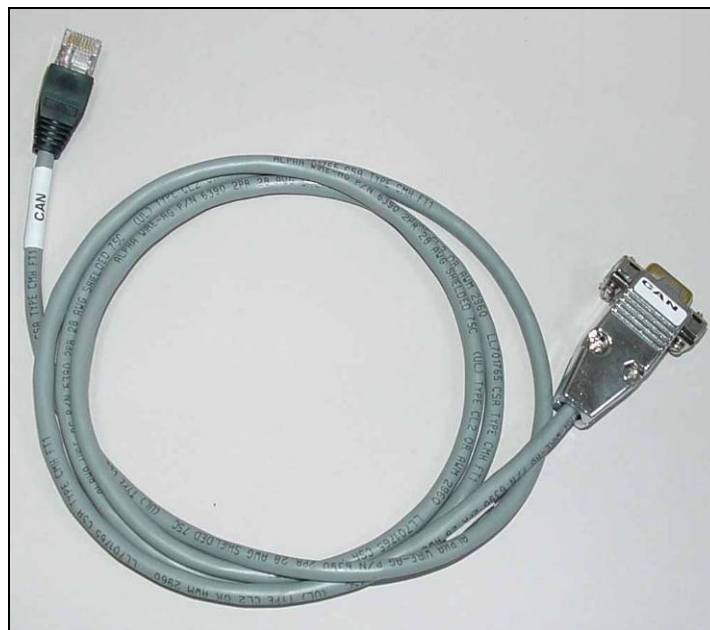
Figure 11: CAN Cable (Part No. CBL-RJ45CAN1-5)
