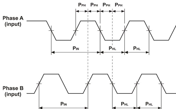
Figure 33: Main Feedback - Encoder Phase Diagram
