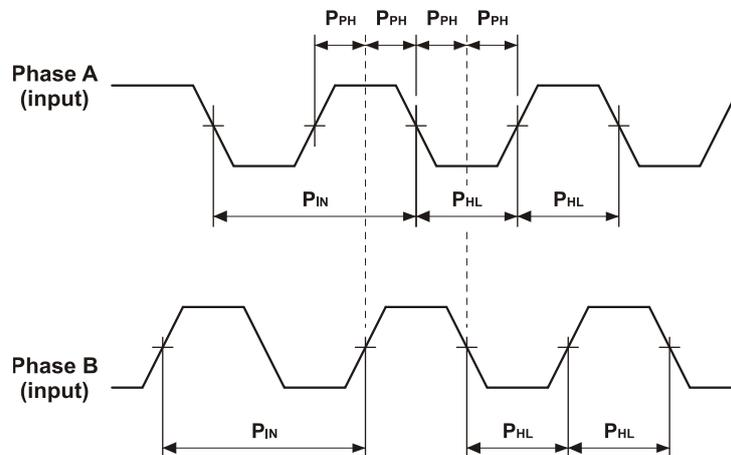
Figure 34: Auxiliary Feedback - Encoder Phase Diagram
