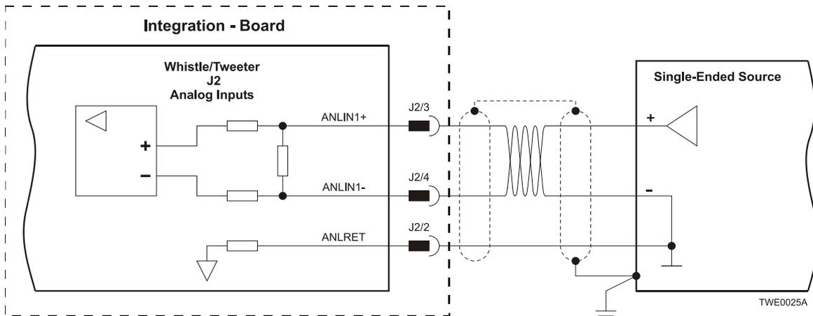
Figure 29: Analog Input with Single-Ended Source
