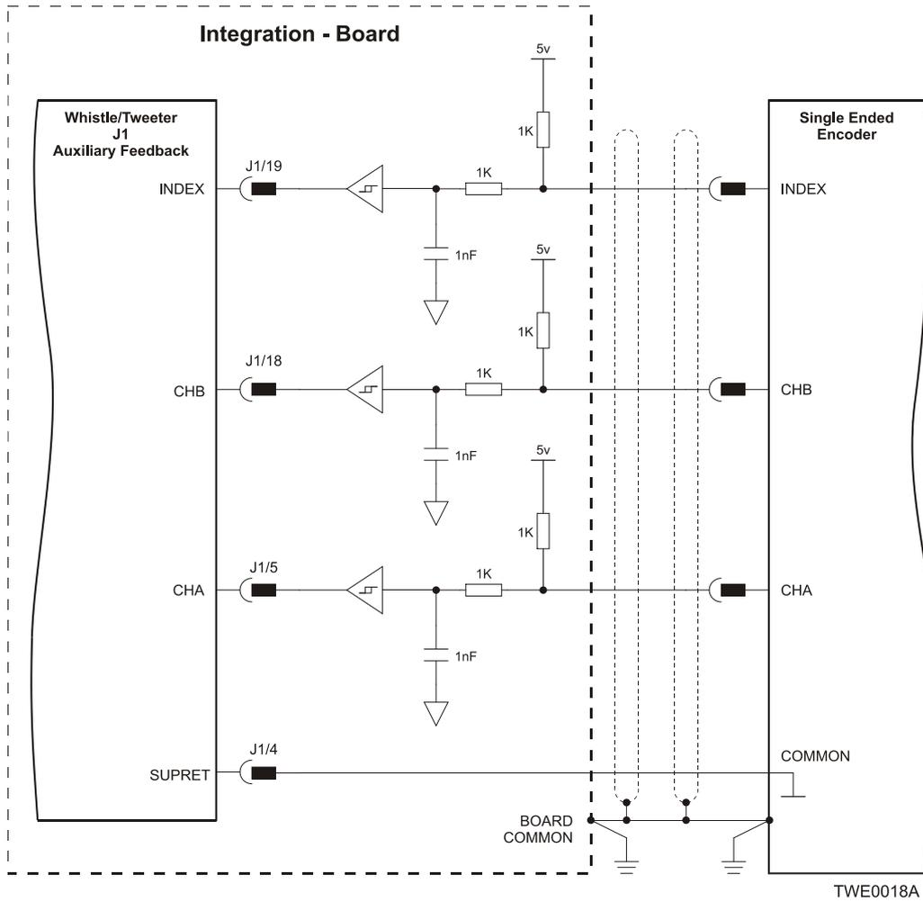
Figure 22: Single-Ended Auxiliary Encoder Input - Recommended Connection Diagram
