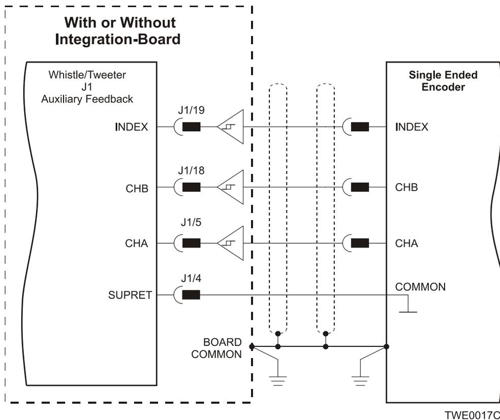
Figure 21: Single-Ended Auxiliary Encoder Input - Acceptable Connection Diagram
