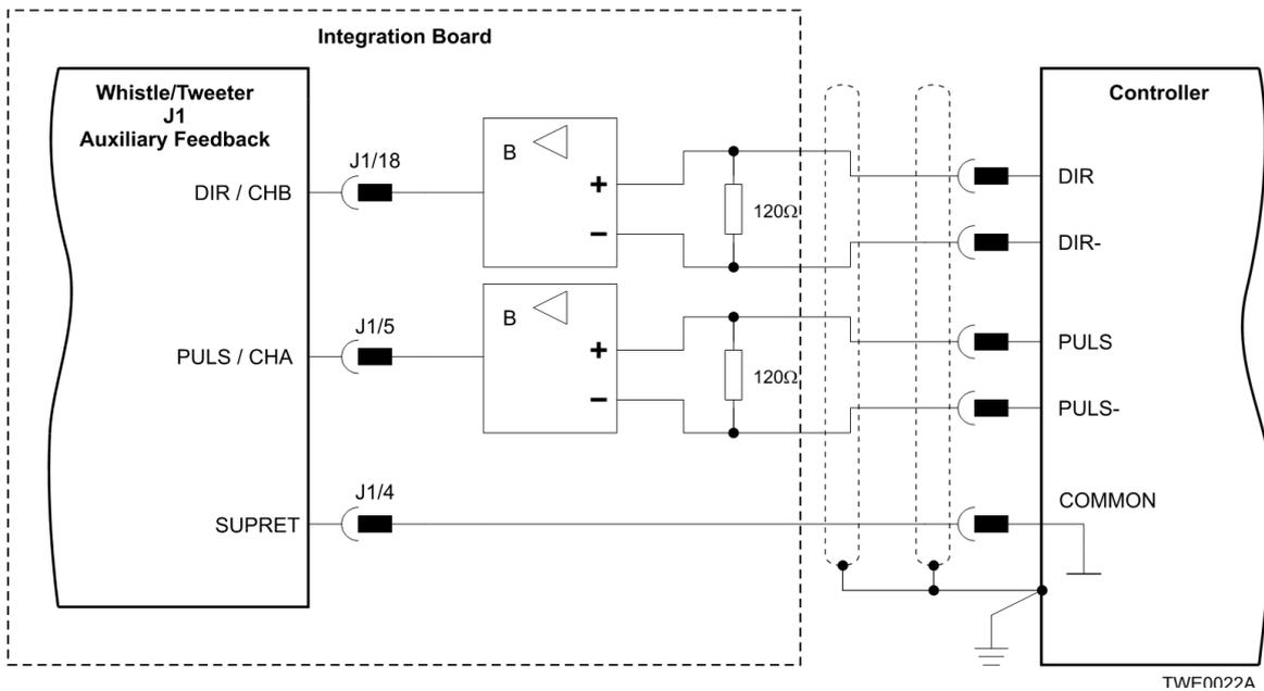
Figure 26: Pulse-and-Direction Auxiliary Encoder Input – Differential Connection Diagram
