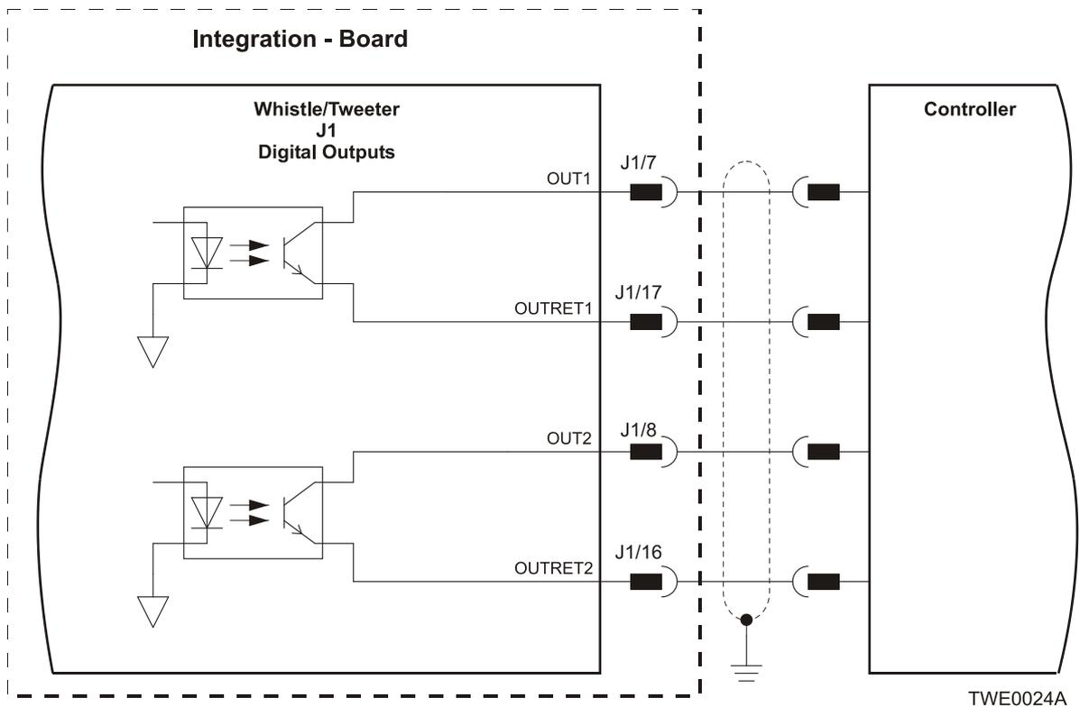
Figure 28: Digital Output Connection Diagram
