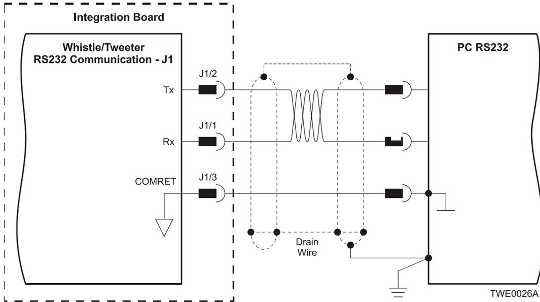
Figure 30: RS-232 Connection Diagram
