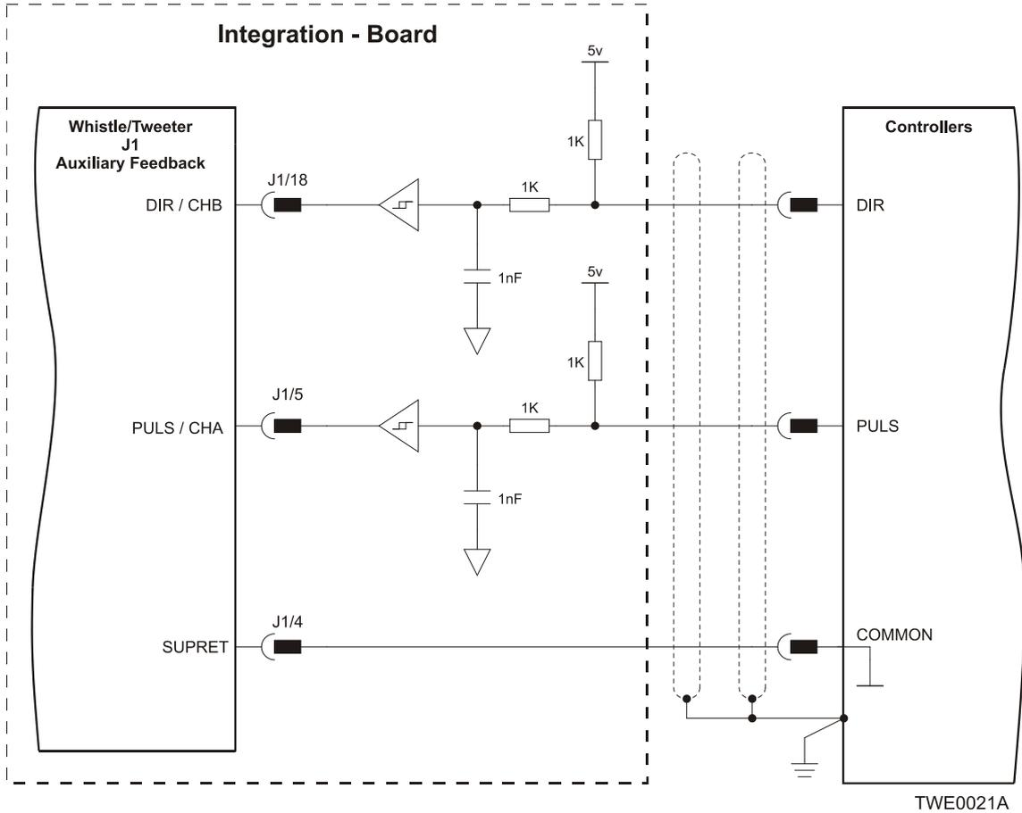
Figure 25: Pulse-and-Direction Auxiliary Encoder Input – Buffered Connection Diagram
