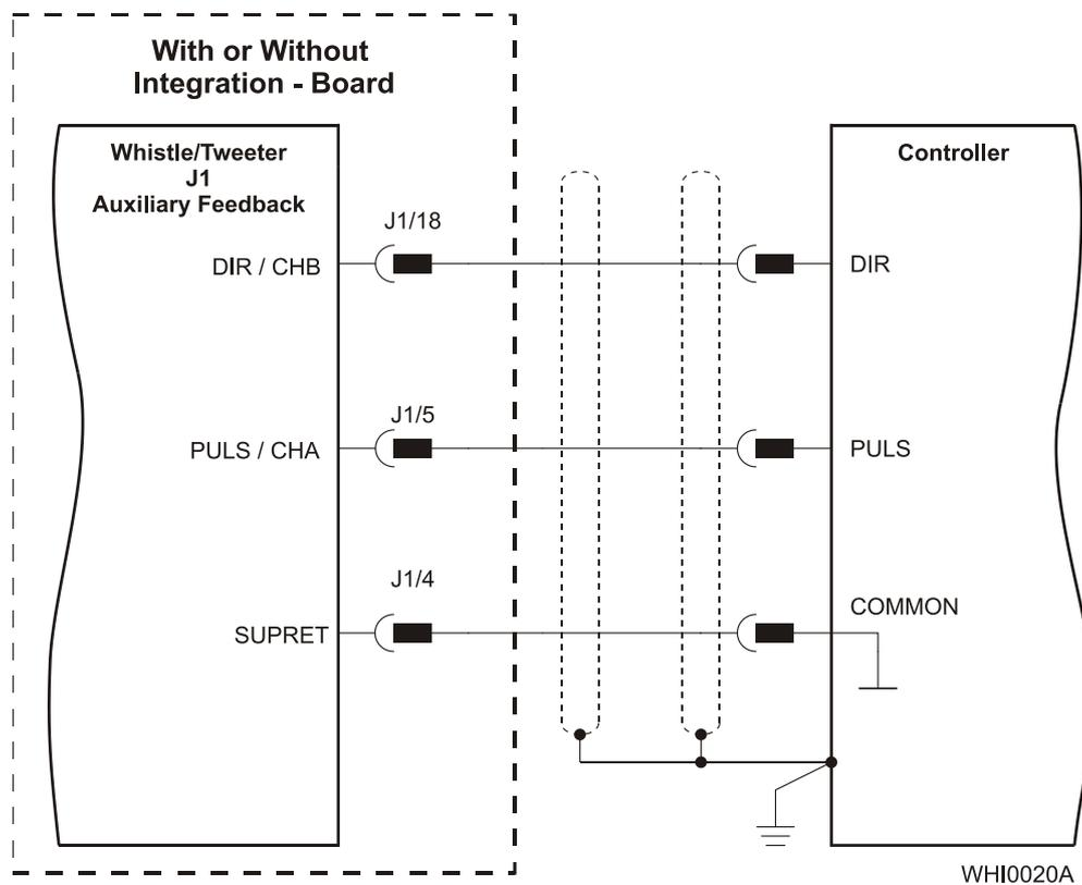
Figure 24: Pulse-and-Direction Auxiliary Encoder Input – Direct Connection Diagram
