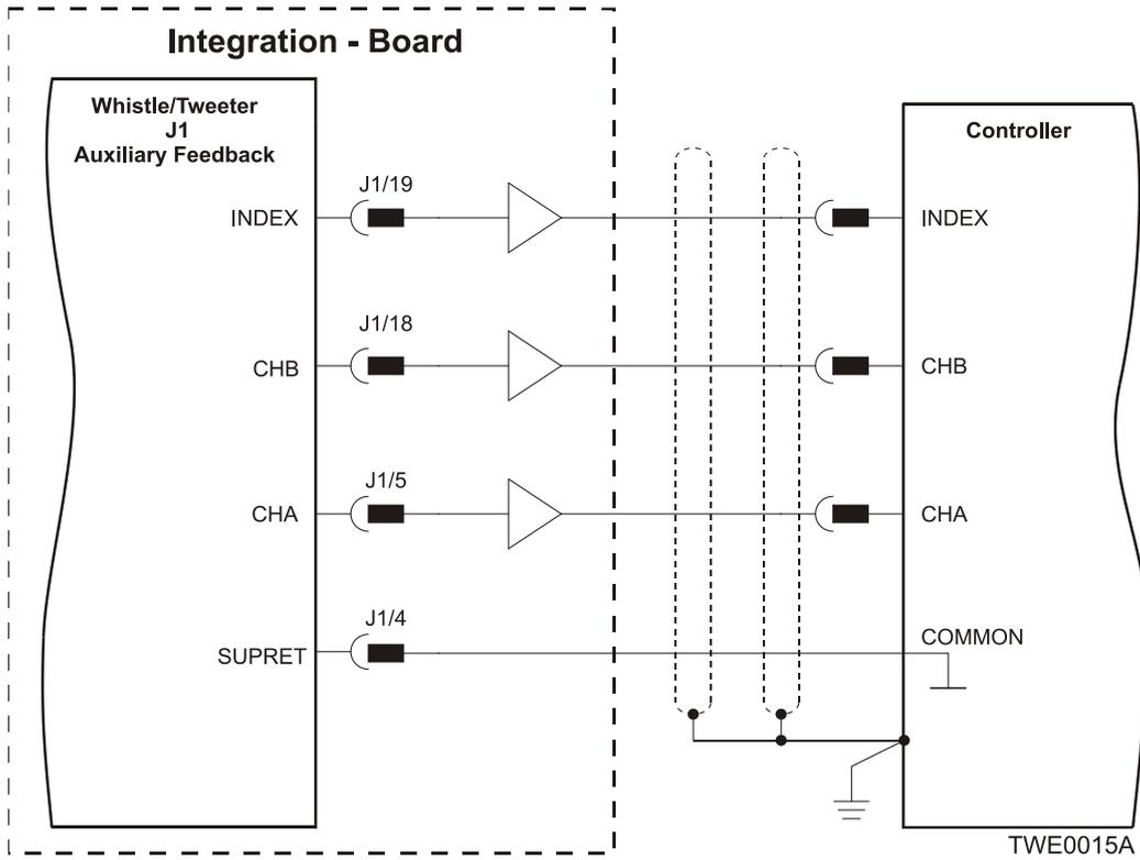
Figure 19: Emulated Encoder Buffered Output – Recommended Connection Diagram
