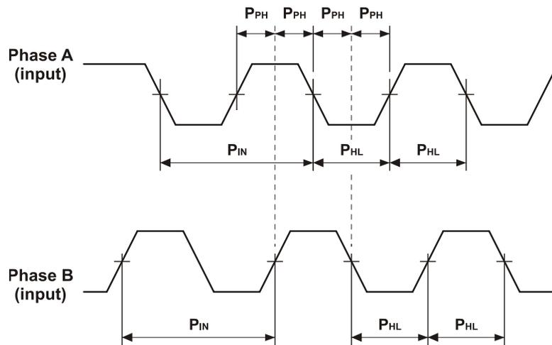
Figure 35: Auxiliary Feedback - Encoder Phase Diagram
