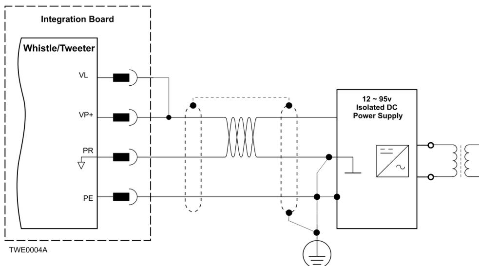
Figure 8: Single Supply for both the Main Power Supply and the Auxiliary Supply in Up to 100 V Models
