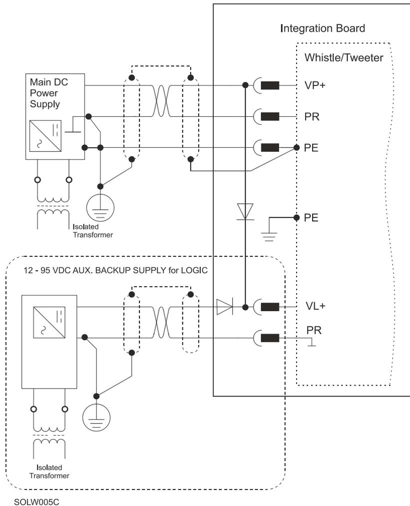
Figure 10: Shared Supply Connection Diagram
