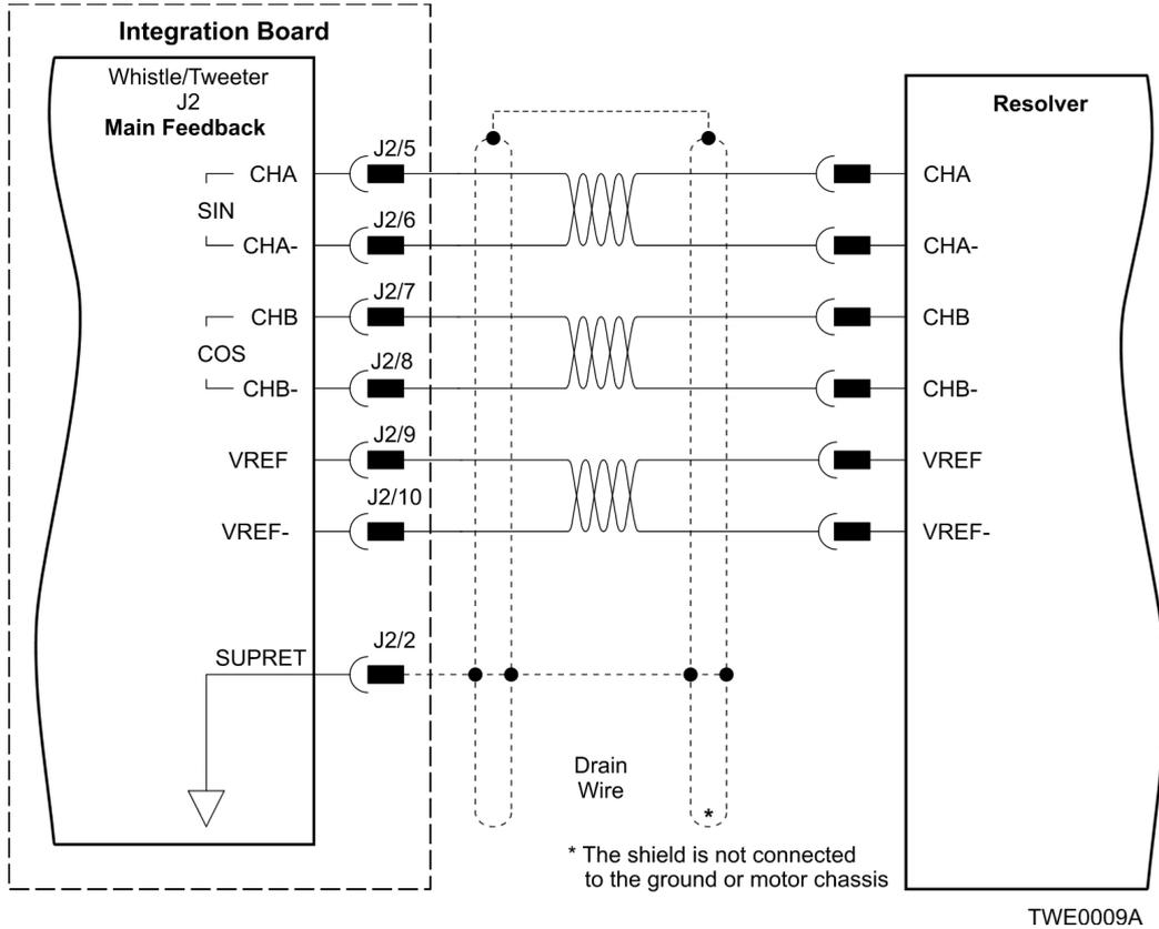
Figure 13: Main Feedback – Resolver Connection Diagram
