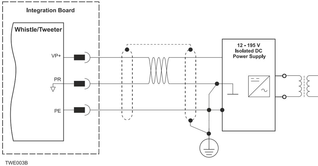
Figure 7: Main Power Supply Connection Diagram
