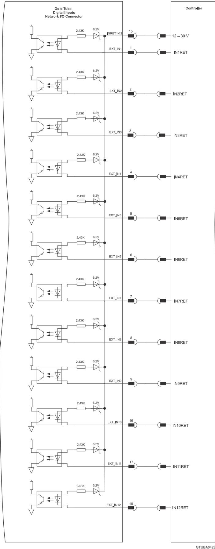
Figure 37: Network I/O Digital Input H Mode Connection Diagram - G-TUBX<sup>XX</sup>/YYYXXHEX
