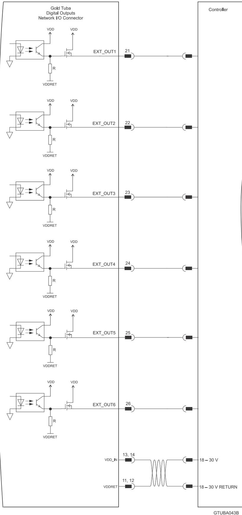
Figure 38: Network I/O Digital Output Connection Diagram – PLC Option, for G-TUB<sub>XX/YYYXXSEX</sub>
