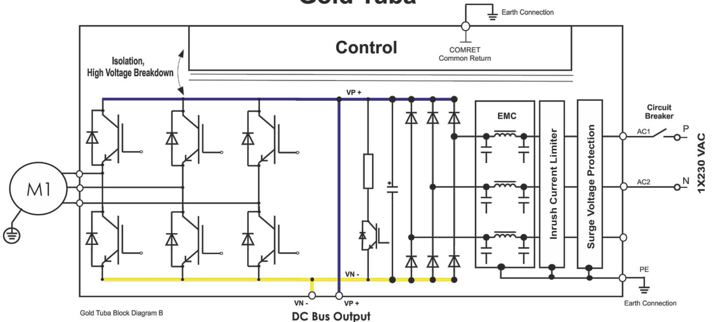
Figure 12: Non-Isolated Single-Phase Source - Connection Topology
