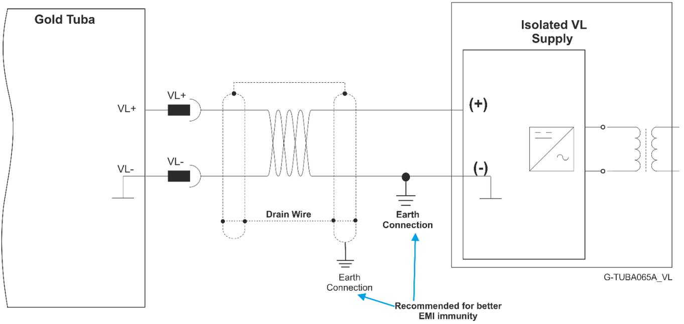
Figure 14: Auxiliary 24 VDC Power Supply Connection Diagram
