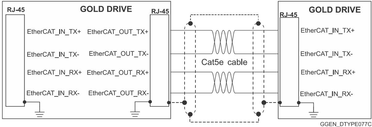
Figure 41: EtherCAT RJ-45 Connections
