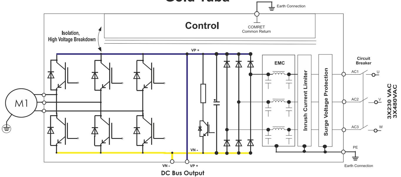
Figure 11: Non-Isolated Three-Phase Source - Connection Topology
