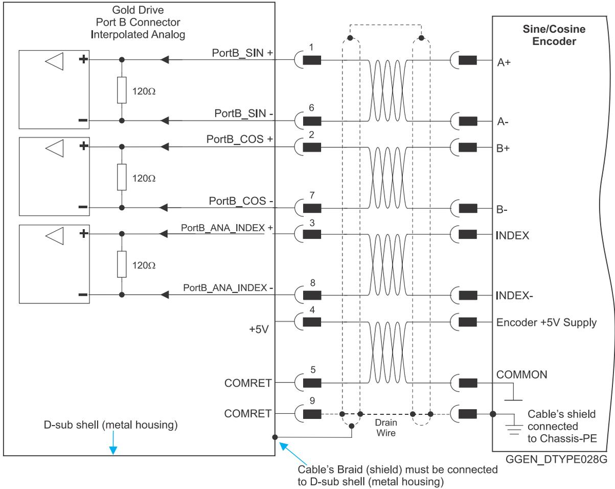
Figure 21: Port B - Interpolated Analog Encoder D-Type Connection Diagram
