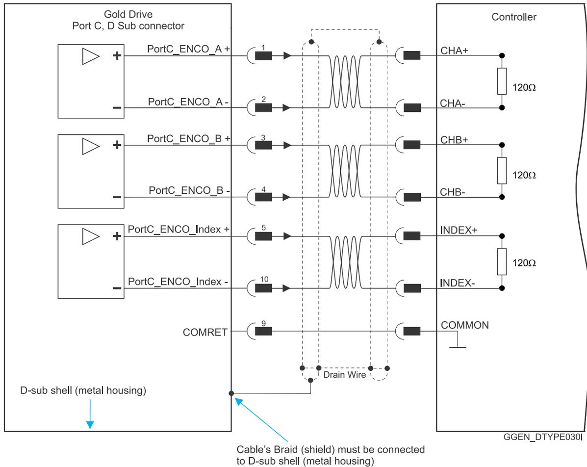
Figure 23: Emulated Encoder Differential Output – Recommended D-Type Connection Diagram
