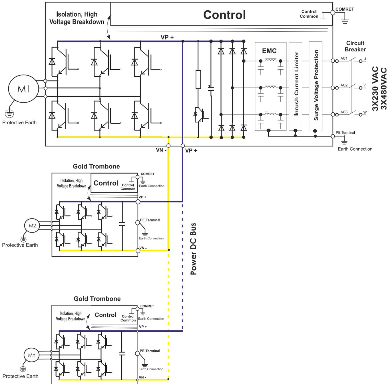
Figure 13: Non-Isolated Three-Phase Source - Multiple Connection Topology
