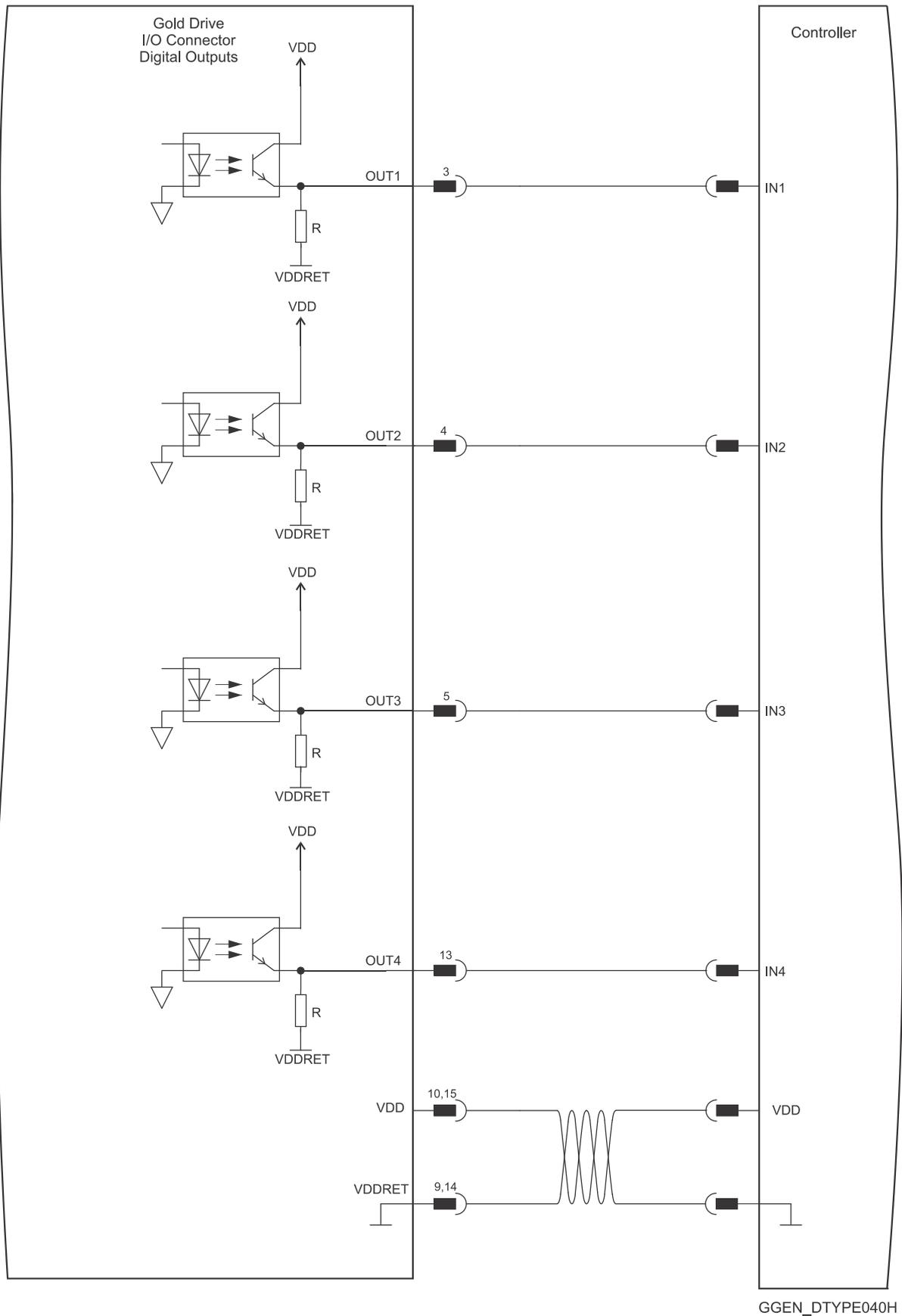
Figure 29: Digital Output D-Type Connection Diagram – TTL Option
