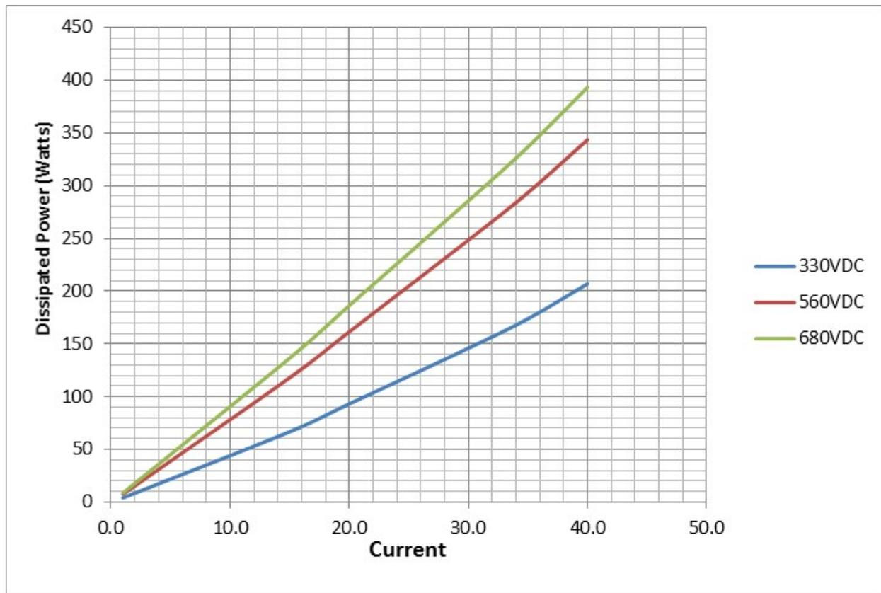
Figure 43: Power Dissipation for Gold Tuba types
