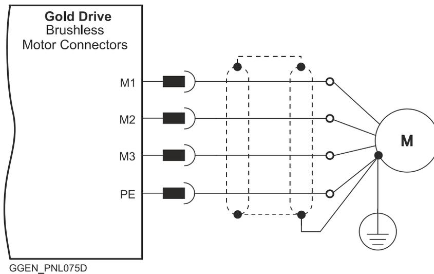
Figure 9: Brushless Motor Power Connection Diagram
