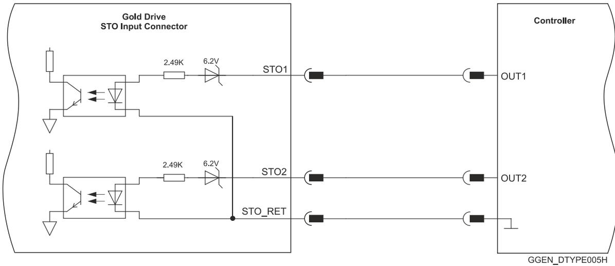
Figure 25: STO Input Connection – PLC Source Option
