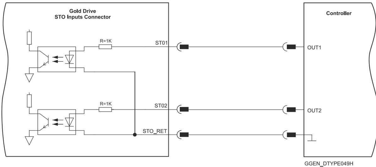
Figure 26: STO Input Connection – TTL Option
