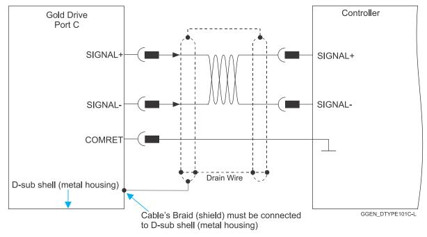
Figure 6: Feedback Port C Cable Assemblies
