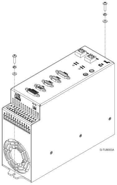
Figure 1: Mounting the Gold Tuba
