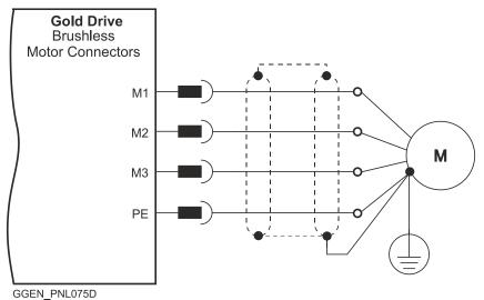
Figure 9: Brushless Motor Power Connection Diagram
