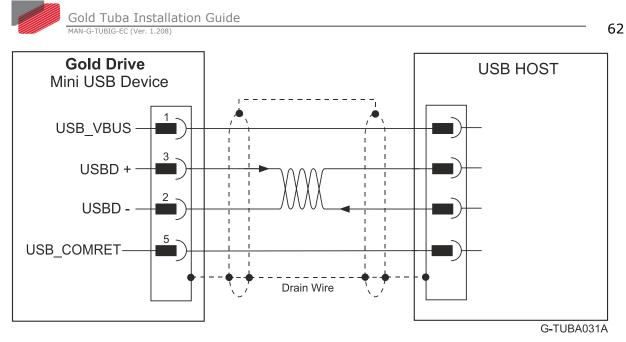
Figure 34: USB Network Diagram
