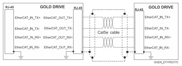
Figure 41: EtherCAT RJ-45 Connections
