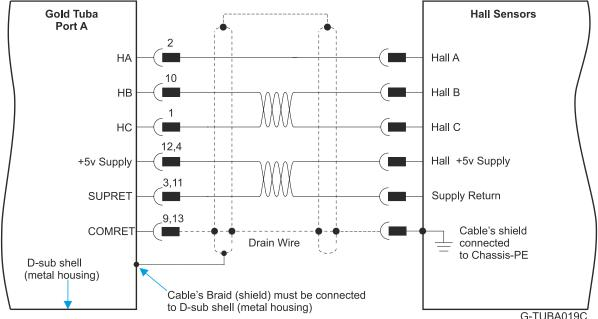
Figure 16: Hall Sensor Connection Diagram
