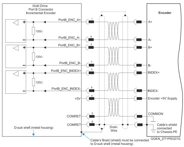
Figure 20: Port B Incremental Encoder Input – Recommended D-Type Connection Diagram
