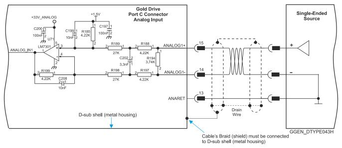
Figure 24: Differential Analog D-Type Input
