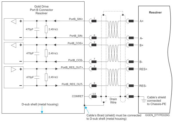
Figure 22: Port B – Resolver D-Type Connection Diagram
