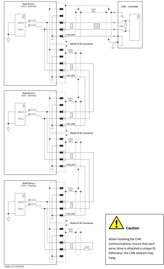
Figure 42: Gold Tuba Connection Diagram – CAN
