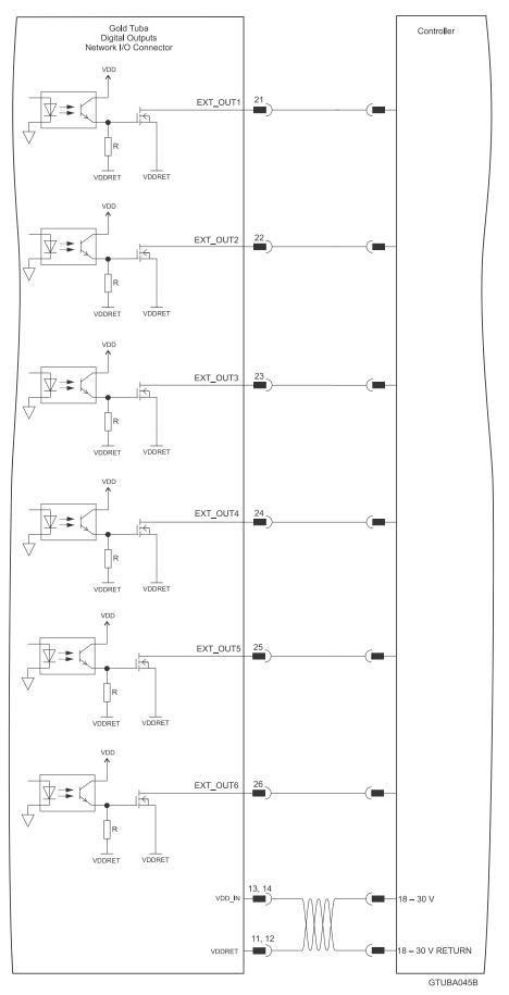
Figure 40: Network I/O Digital Output Connection Diagram – H Option - G-TUBXXX/YYYXXHEX
