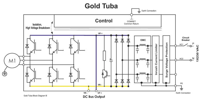
Figure 12: Non-Isolated Single-Phase Source - Connection Topology
