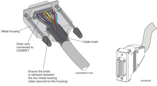
Figure 4: D-Type Cable Assemblies
