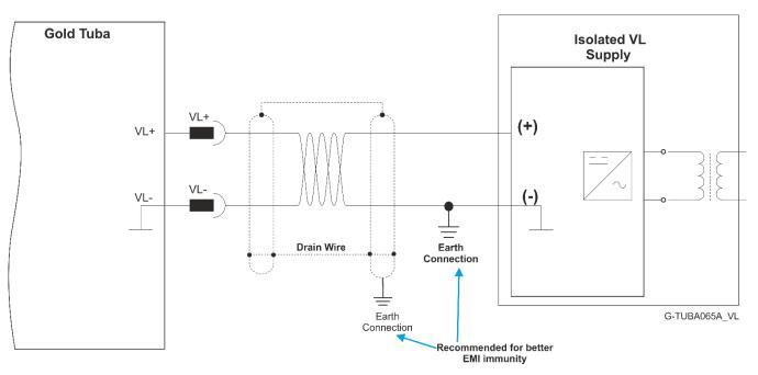
Figure 14: Auxiliary 24 VDC Power Supply Connection Diagram
