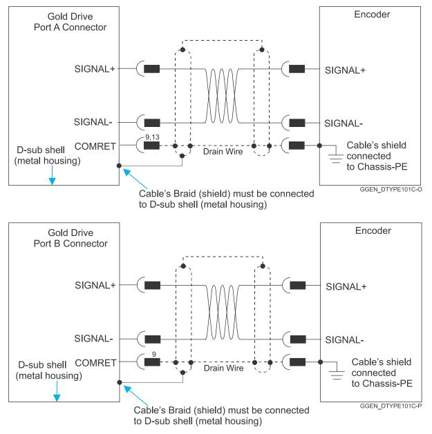
Figure 5: Feedback Port A and B Cable Assemblies
