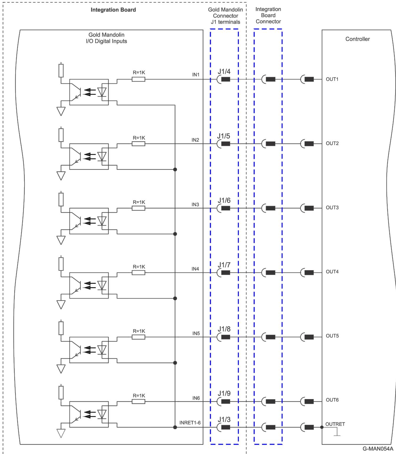
Figure 30: Digital Input TTL Mode Connection Diagram
