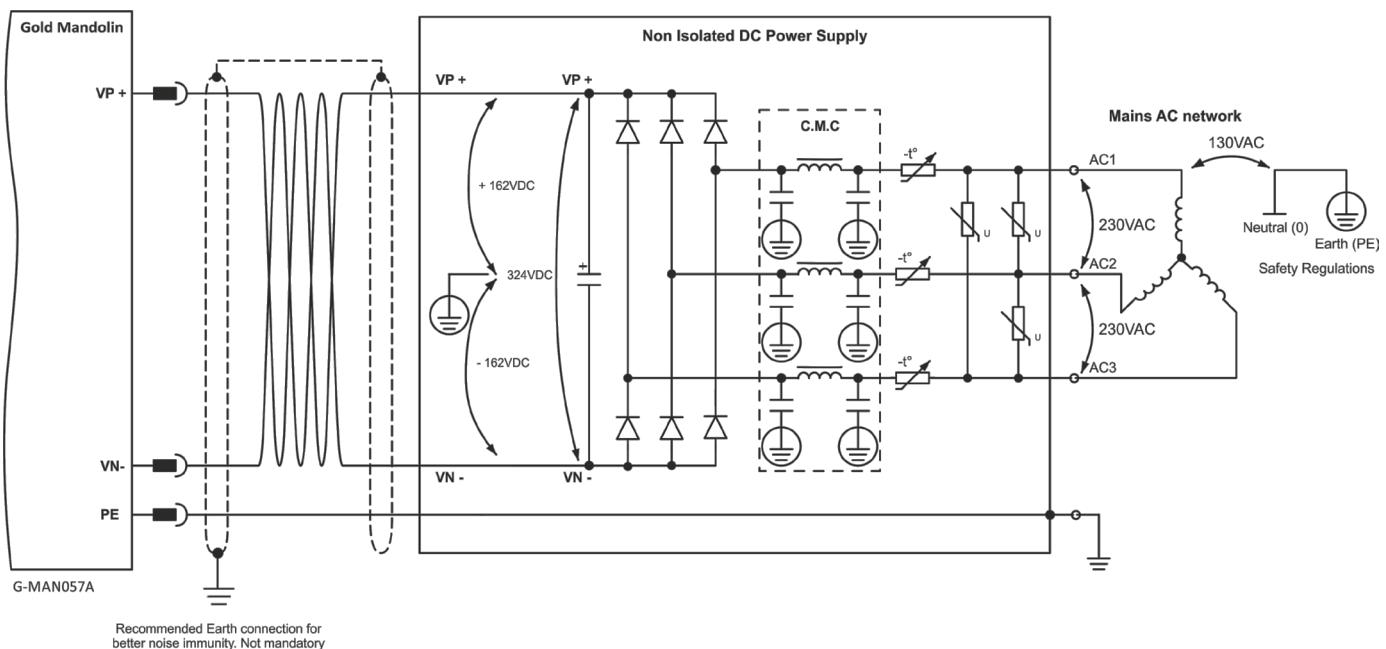
Figure 8: Non-Isolated Three-Phase Connection Topology
