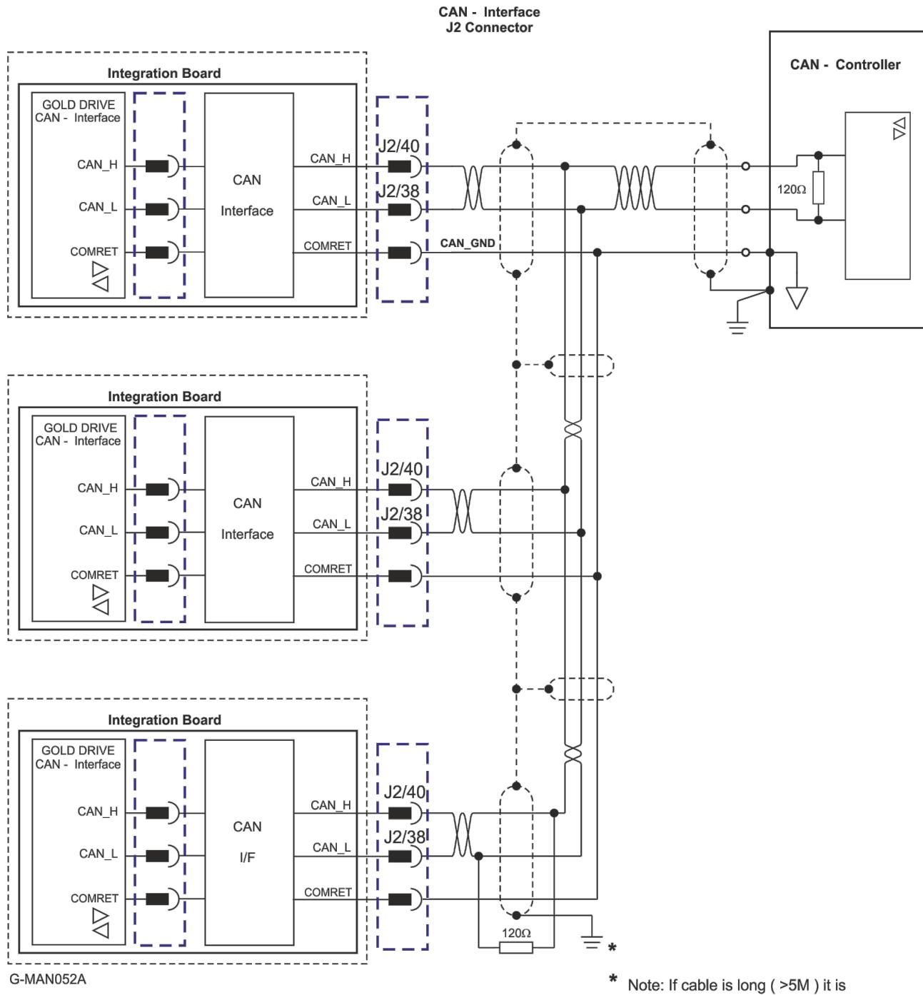
Figure 29: CANbus Connections
