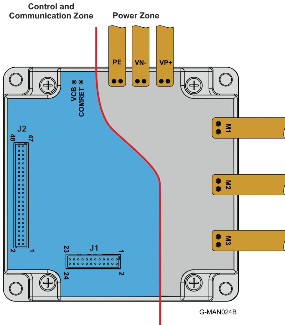
Figure 3: Gold Mandolin Power Conductors PCB layout
