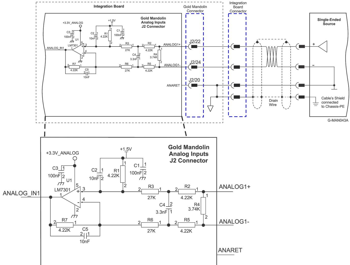
Figure 24: Analog Input with Differential  $\pm 10$  V
