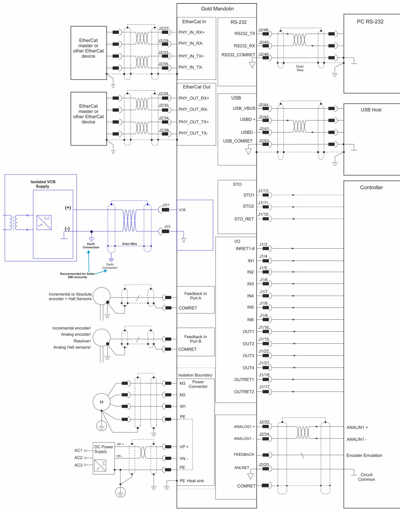
Figure 4: Gold Mandolin Connection Diagram for EtherCAT
