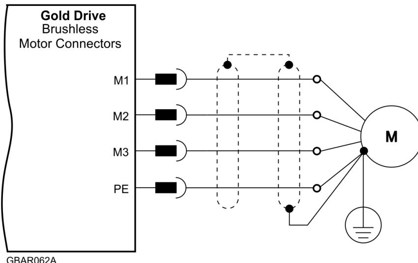
Figure 6: Brushless Motor Power Connection Diagram
