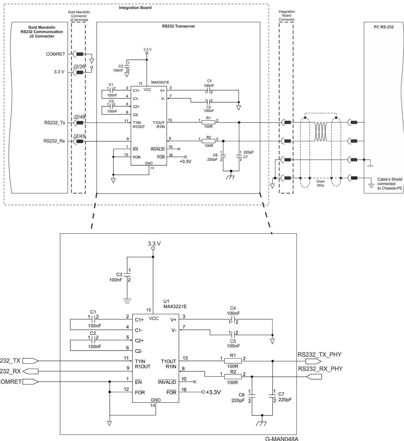
**Figure 26: Standard RS232 Voltage Level incorporating RS232 TX/RX Transceiver Connection Diagram**
