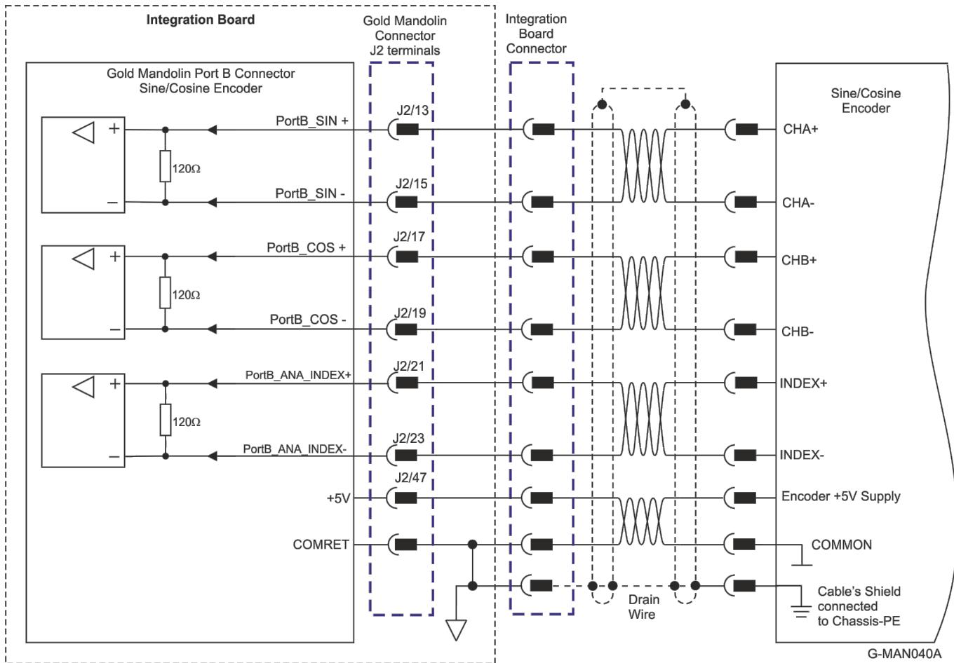
Figure 21: Port B - Interpolated Analog Encoder Connection Diagram
