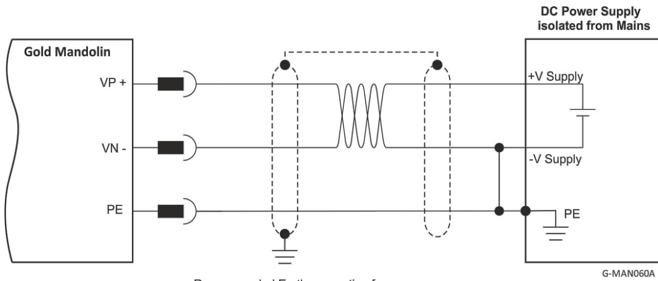
Figure 11: Battery Connection Topology
