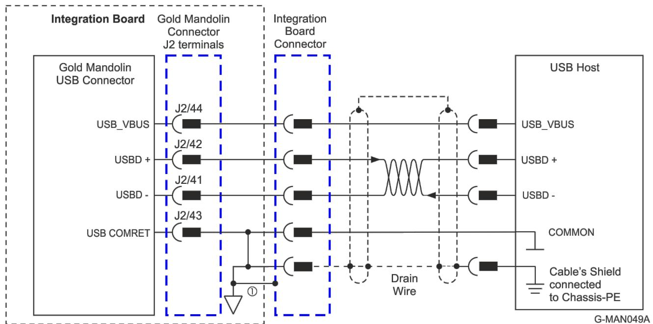
Figure 27: USB Network Diagram
