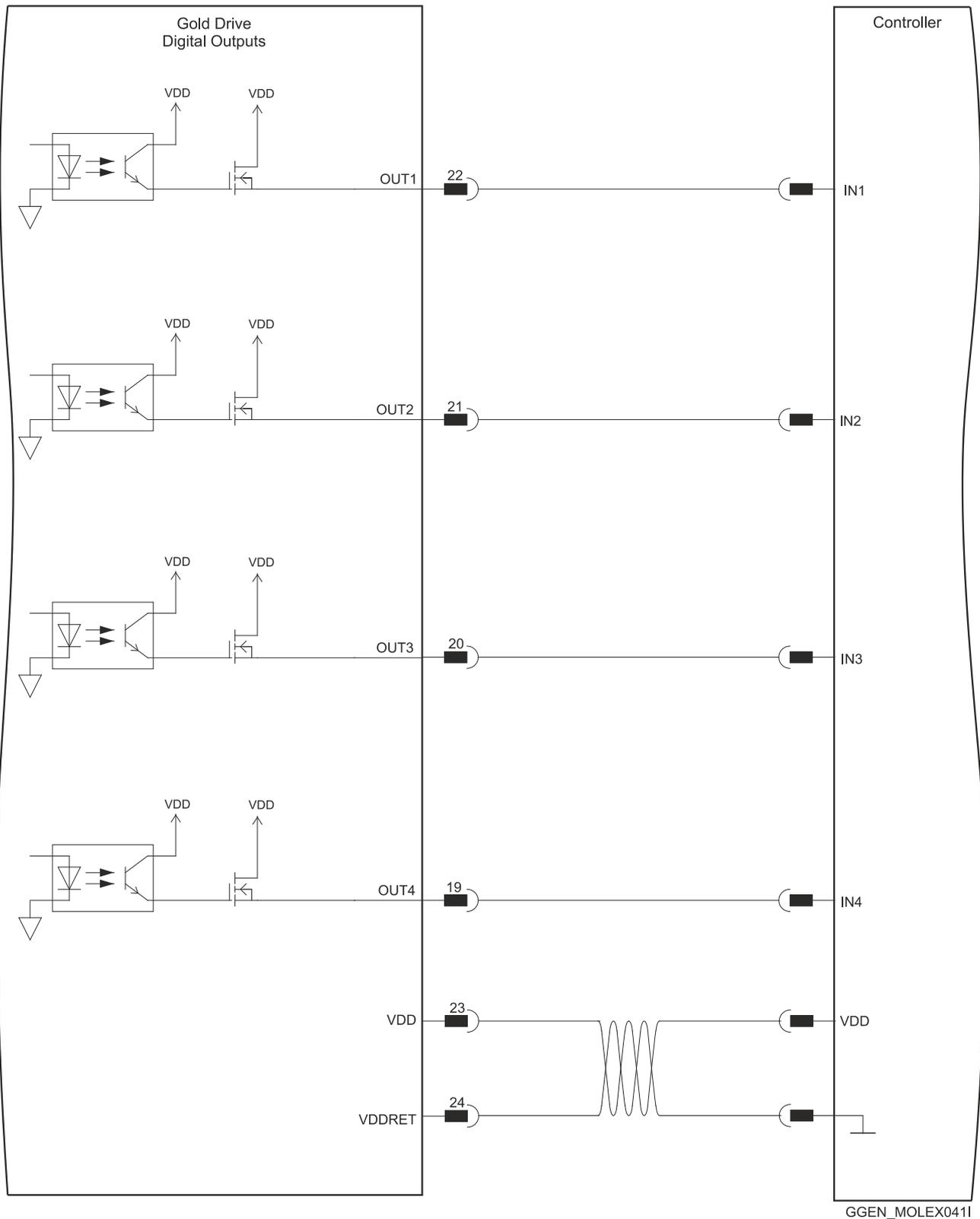
Figure 33: Digital Output Connection Diagram – Source PLC Option
