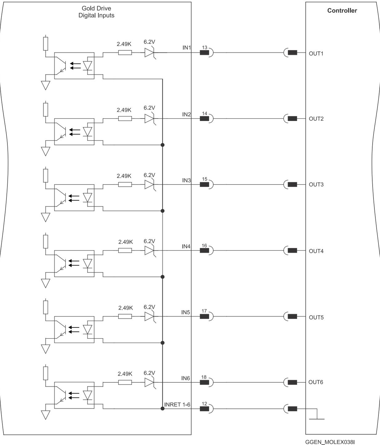
Figure 32: Digital Input Connection Diagram – Source PLC Option
