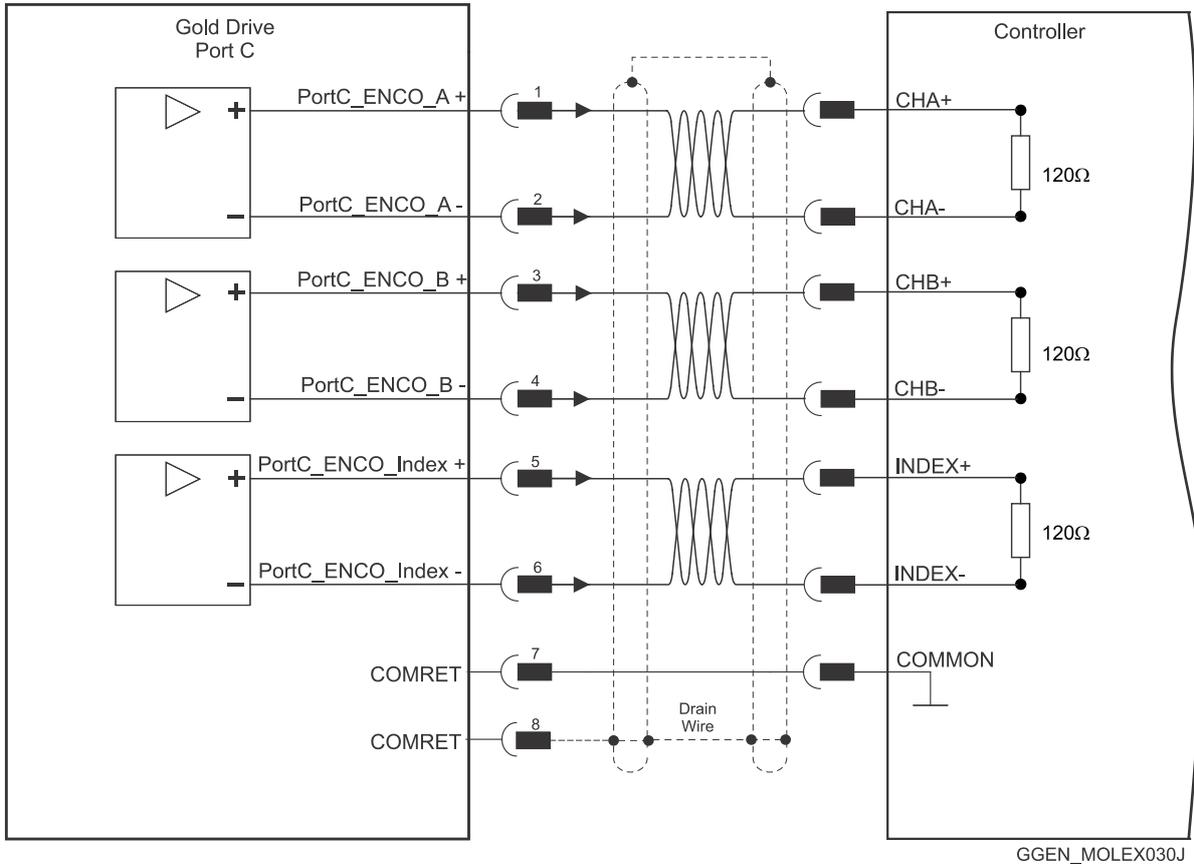
**Figure 28: Emulated Encoder Differential Output – Recommended Connection Diagram**
