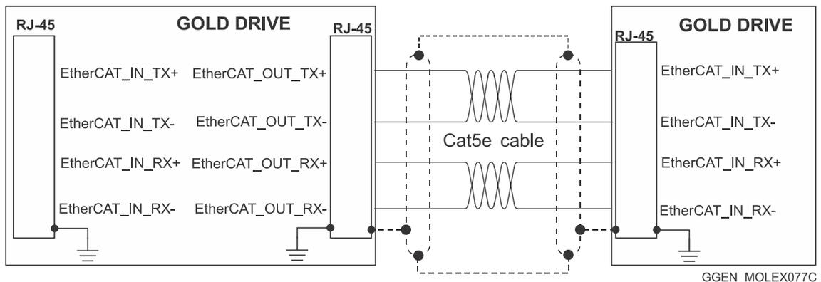
Figure 37: EtherCAT RJ-45 Connections
