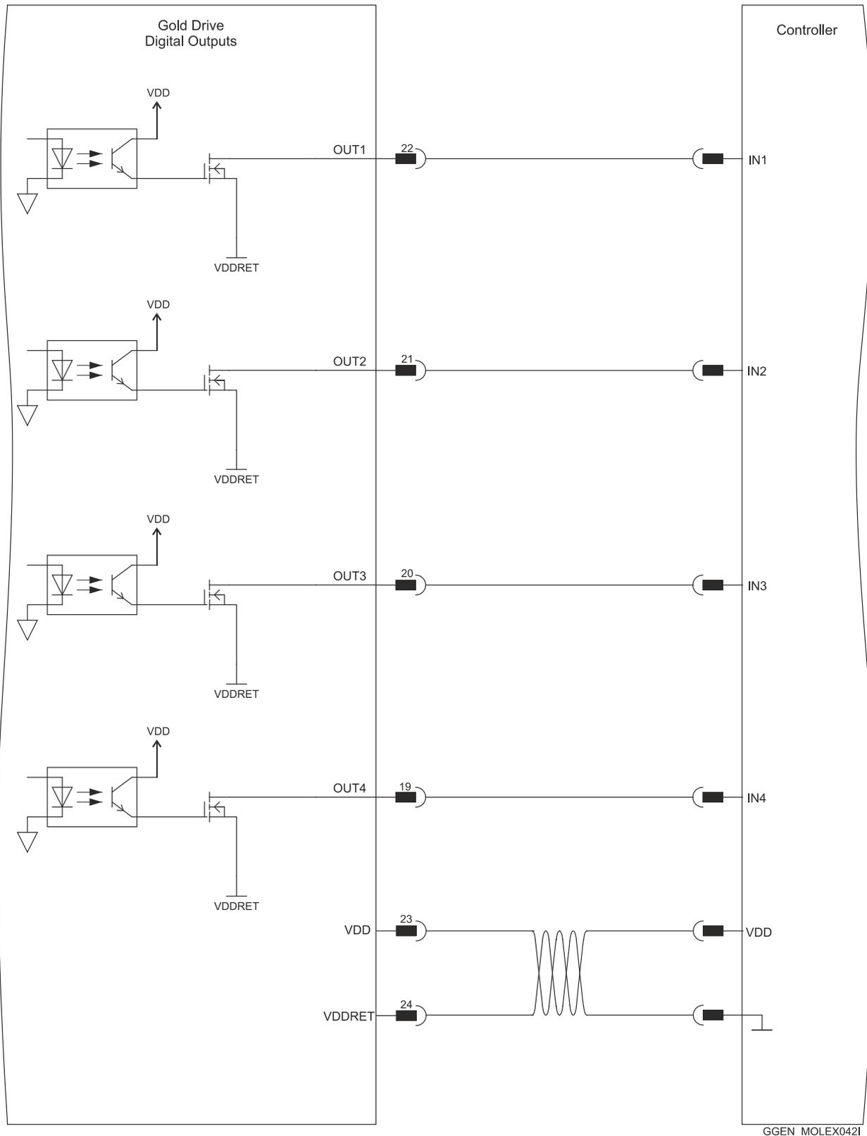
**Figure 35: Digital Output as Sink Configuration Molex Type Connection Diagram**
