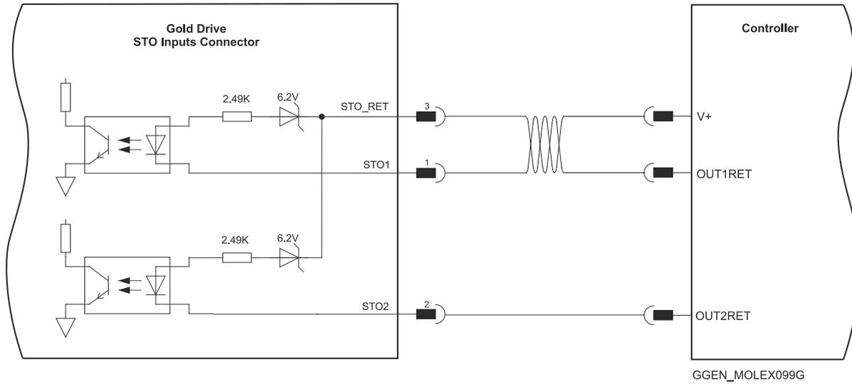
Figure 19: STO Input Connection – Sink Option
