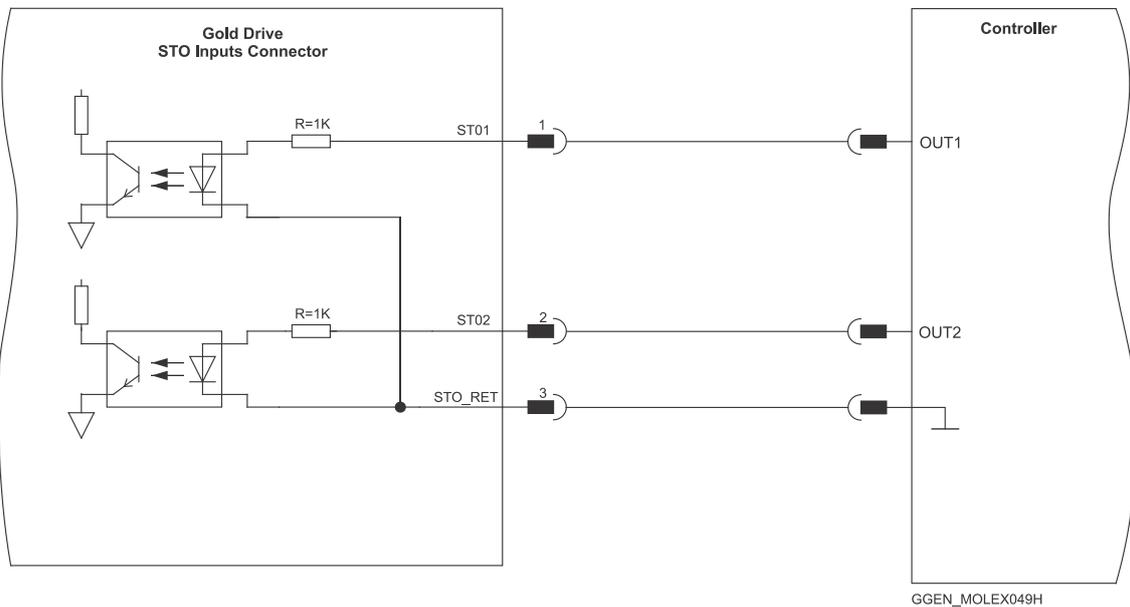
Figure 18: STO Input Connection – TTL Option
