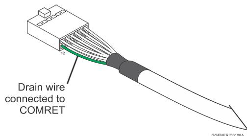
Figure 4: Feedback and Molex Control Cable Assemblies
