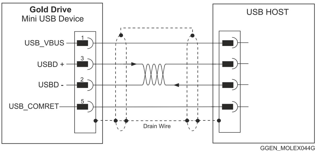
Figure 36: USB Network Diagram
