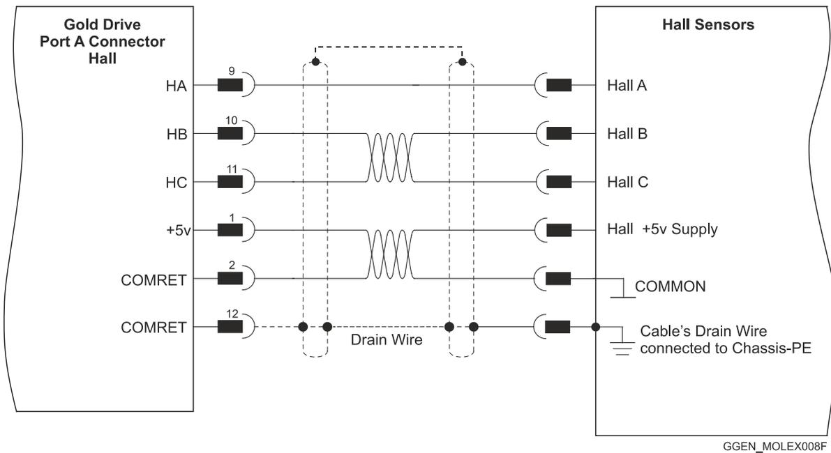
Figure 21: Molex Type Hall Sensors Connection Diagram
