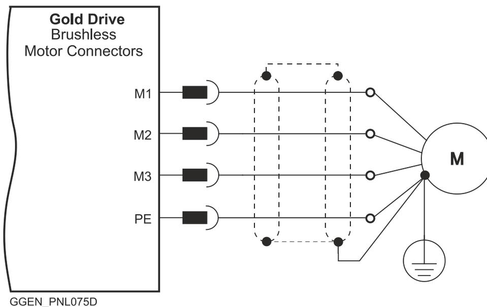
Figure 10: Brushless Motor Power Connection Diagram
